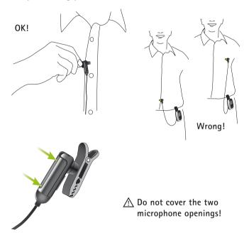
If you are uncertain whether the iLapel is in the correct position, activate the SoundCheck feature in inspiro. SoundCheck helps to position the iLapel correctly.
