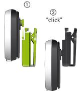
Attach the clip to the button on the backside of the inspiro. Make sure the clip holds securely on the inspiro.
