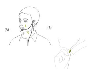
Make sure the head of the microphone is well positioned, as depicted on page 21 (A). If required you can easily bend the boom part (B).
