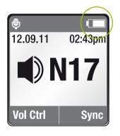
If the charging unit is removed from the inspiro, the battery symbol shows the actual capacity.
